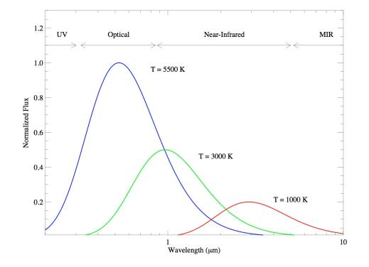
For lowest T<sub>eff</sub> peak flux moves toward infrared wavelengths (Wein's Law), optical flux minimal.
