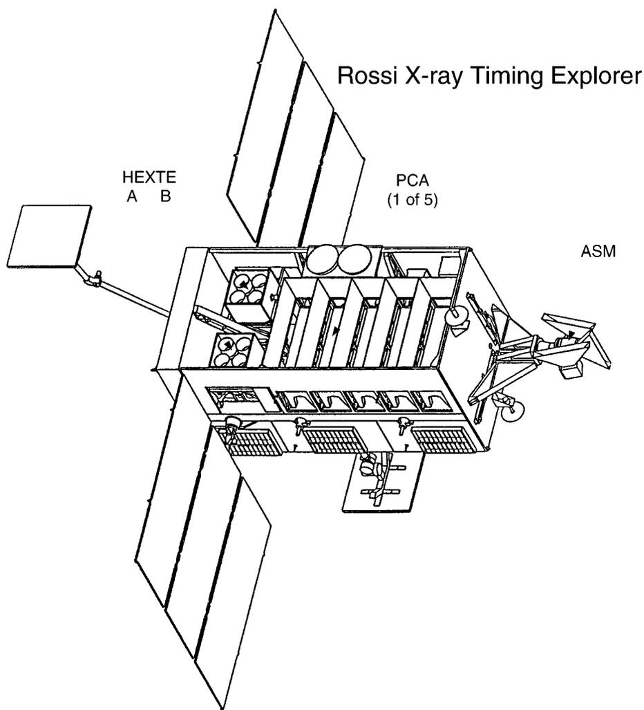
FIG. 1.—RXTE spacecraft viewed from above to reveal the scientific instruments. The five PCA proportional counters and the two HEXTE clusters are shown in relation to the rest of the spacecraft components, such as the two high gain antennae for communications with the ground via the tracking and data relay satellite system, the two solar-power arrays that can rotate to face the Sun, and the ASM on the end with clearance to view the sky.
