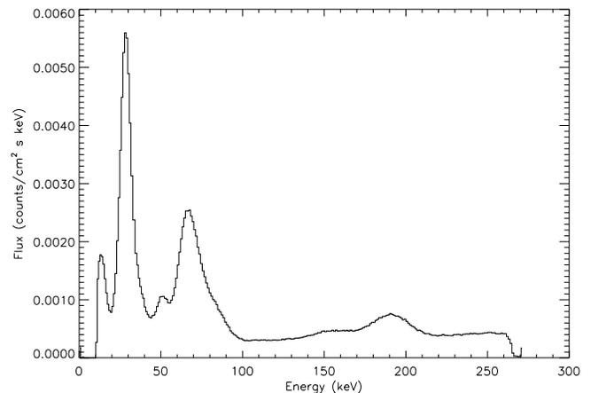
FIG. 6.—HEXTE background for a single detector plotted versus energy. Background lines due to activation of the iodine by cosmic and trapped radiation are evident at 30, 55, 66, and  $\sim 190$  keV, as are the  $K_{\alpha,\beta}$  lines at 74 and 85 keV from fluorescence of the lead collimator. The data are from a 7.5 hr observation of blank sky fields.
