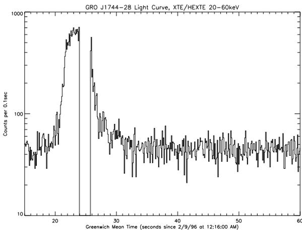
FIG. 13.—Light curve of the bursting pulsar 1744–28 taken during the in-orbit checkout phase of the *RXTE* mission. Individual pulses at the 2.1 Hz pulse period are evident in the persistent flux and a burst is also evident. The less than 2 s dropout and recovery of data during the burst were caused when X-ray rates exceeded the maximum transferable rate.
