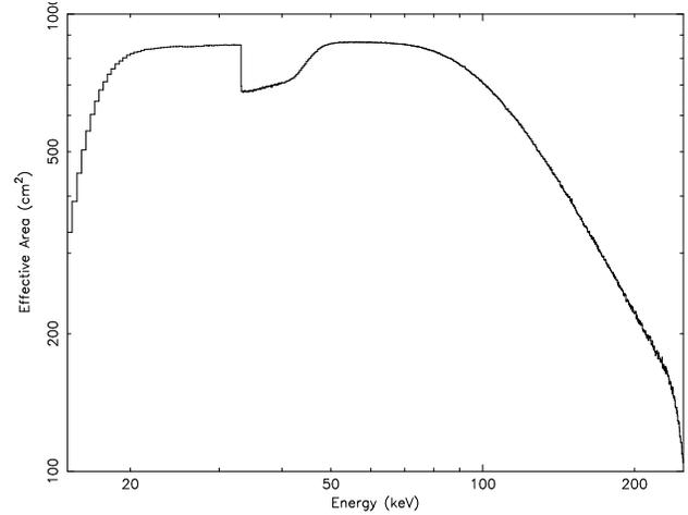
FIG. 5.—HEXTE effective area versus energy for cluster A. The reduction at lower energies is due to photoelectric absorption in the housing above the detector, while the reduction at higher energies is due to the finite NaI(Tl) thickness. The sharp drop and smooth recovery near 30 keV is due to the change in photoelectric cross section at the K edge of iodine and the onset of K-escape losses.
