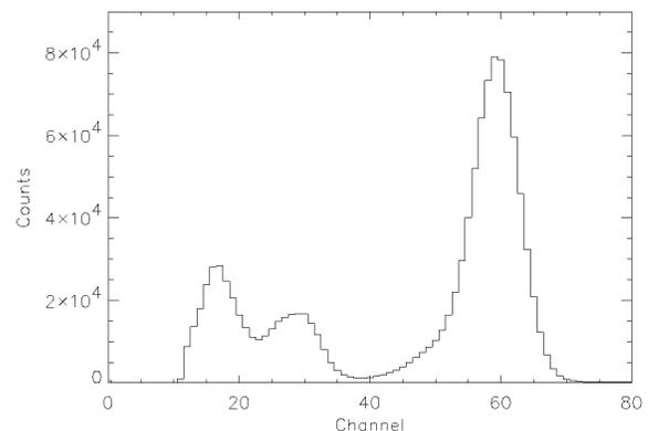
FIG. 3.—Calibration histogram of the HEXTE  $^{241}\text{Am}$  gain control source. The data were accumulated over one day on 1997 January 10. The 60 keV gamma-ray line, the complex of Np L de-excitation lines around 17 keV, and the K-escape lines near 30 keV are evident. Each channel corresponds to approximately 1 keV.
