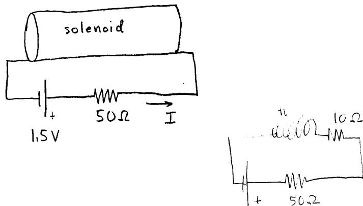
Assume that the solenoid itself has an additional small resistance of  $10\Omega$ . What is the magnitude of the magnetic field inside of the solenoid?
