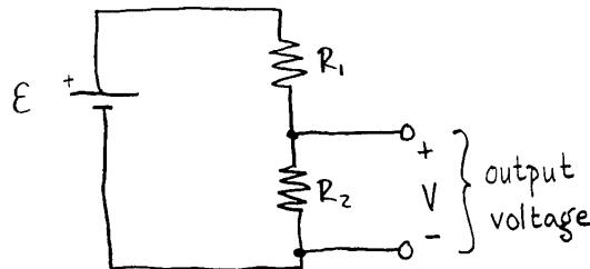
(a) What is the output voltage,  $V$ , in terms of  $R_1$ ,  $R_2$ , and the *emf*? (15 pts)
