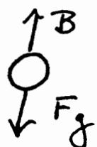
$F_g = mg = \rho V g$  acting downward on the volume. If it is not falling then there must be a force opposing
