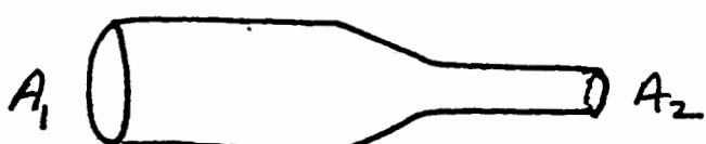
If we introduce fluid into  $A_1$  with velocity  $v_1$ , then the eqn of continuity requires
