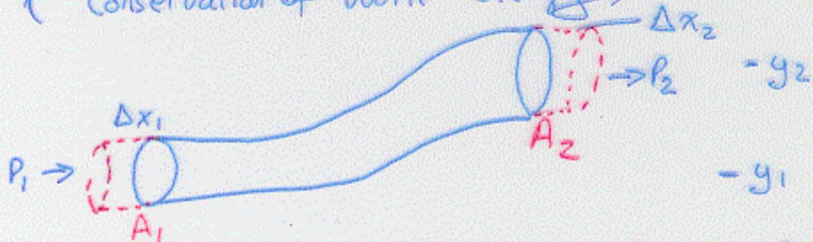
In time  $\Delta t$ , mass  $m$  of fluid travels  $\Delta x_1 = V_1 \Delta t$
