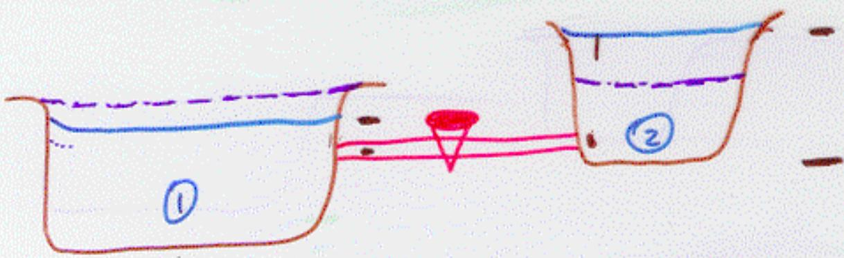
Open valve in pipe: higher pressure in ② forces liquid from ② to ① until each end of pipe is at same pressure, i.e. same depth
