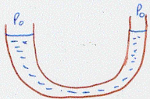
level does not depend on width of tube.
