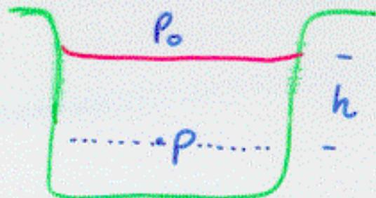
$P_0 = \text{atm. pressure at surface} = \text{weight of air column}$
