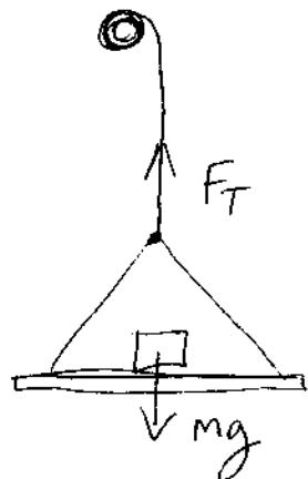
For elevator mass  $M$
