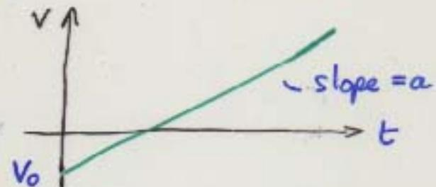
And position  $x(t) = \int v \cdot dt = x_0 + \int_0^t \underline{(v_0 + at)} \cdot dt$
