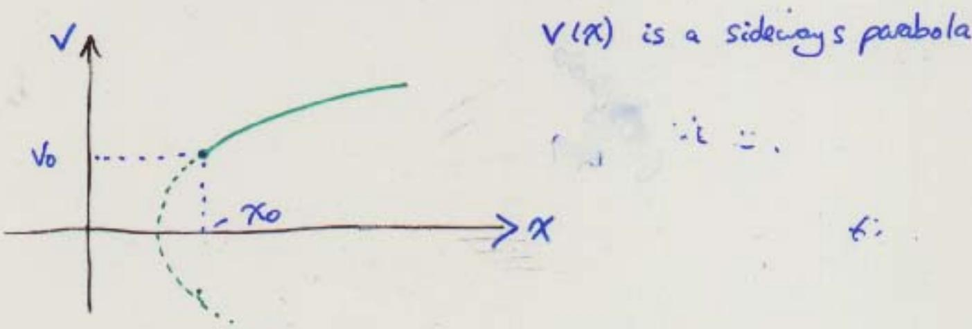
Note: Be careful with sign of  $v = \pm \sqrt{v_0^2 + 2a(x - x_0)}$
