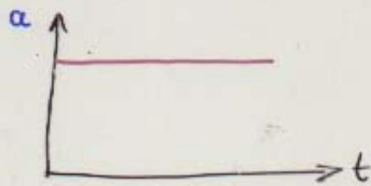
Then speed  $v = \int a \cdot dt = v_0 + \int_0^t a \cdot dt = v_0 + at$
