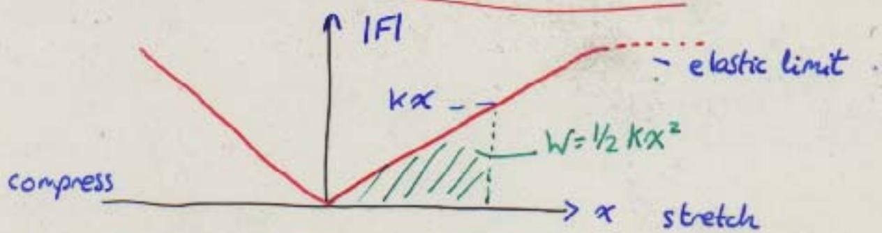
Most springs, wires obey Hooke's law up to an elastic limit
