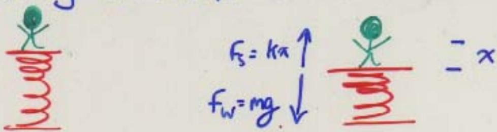
Scale drops to new eqm. position  $F_s = F_w \Rightarrow x = \frac{mg}{k} = 0.25\text{m}$
