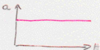
$$\text{Then } v = \int a \cdot dt = v_0 + \int_0^t a \cdot dt = v_0 + at$$
