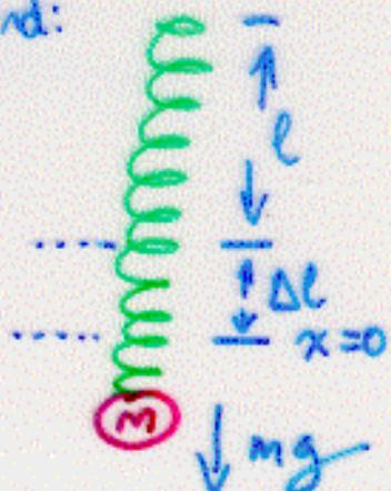
1. New eqm. length is where  $k\Delta l = mg$  i.e.  $\Delta l = \frac{mg}{k} = \frac{10 \times 0.5}{10} = 0.5 \text{ m}$
