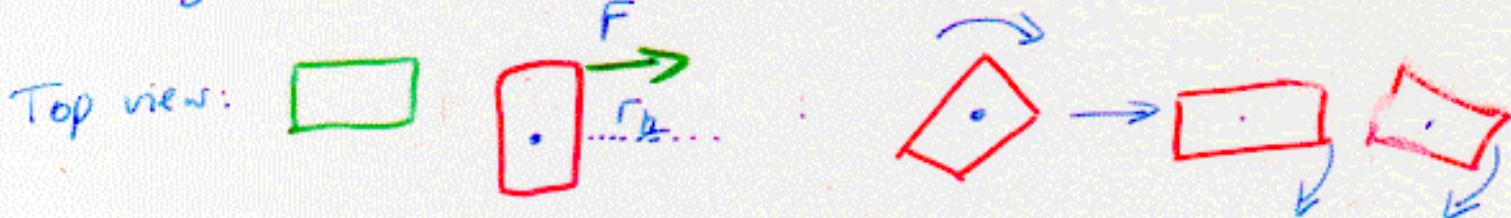
c.f. Force applied with  $r_L = 0$  (in line with c.m.)
