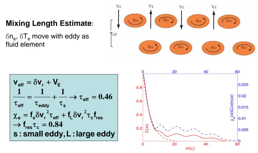
• Large eddies contribute significantly to e transport since electron can travel long distance --- this is essential to produce smooth radial profile of e heat transport
