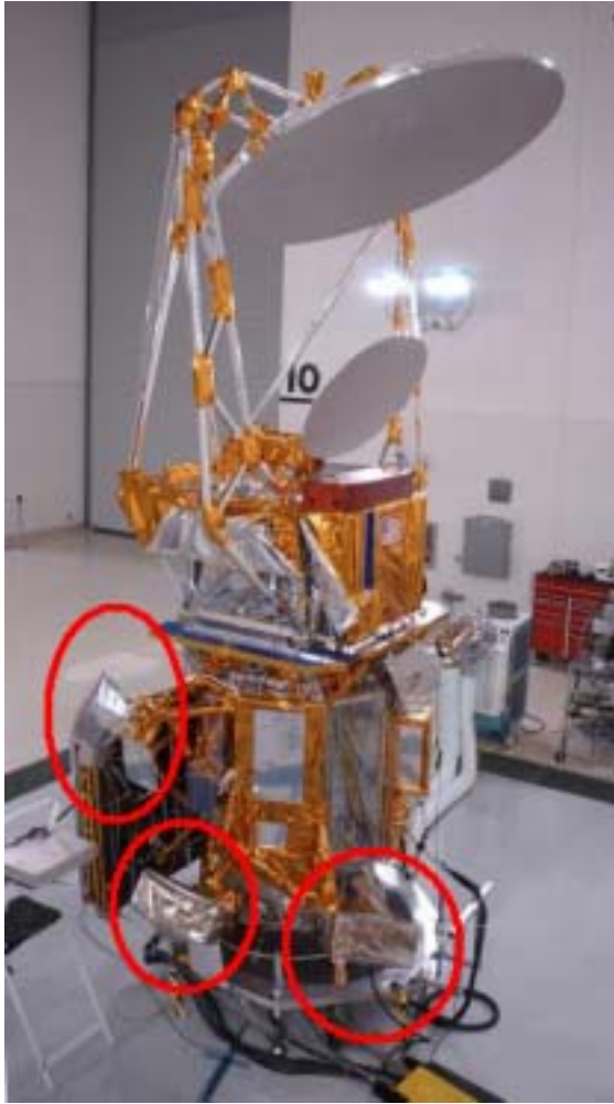
Figure 1 (a) Coriolis spacecraft with the Solar Mass Ejection Imager (SMEI) instrument on board prior to launch. The three instrument camera baffles (circled). (b) Titan II launch of the Coriolis spacecraft on 6 January 2003 with on board SMEI and WindSat.
