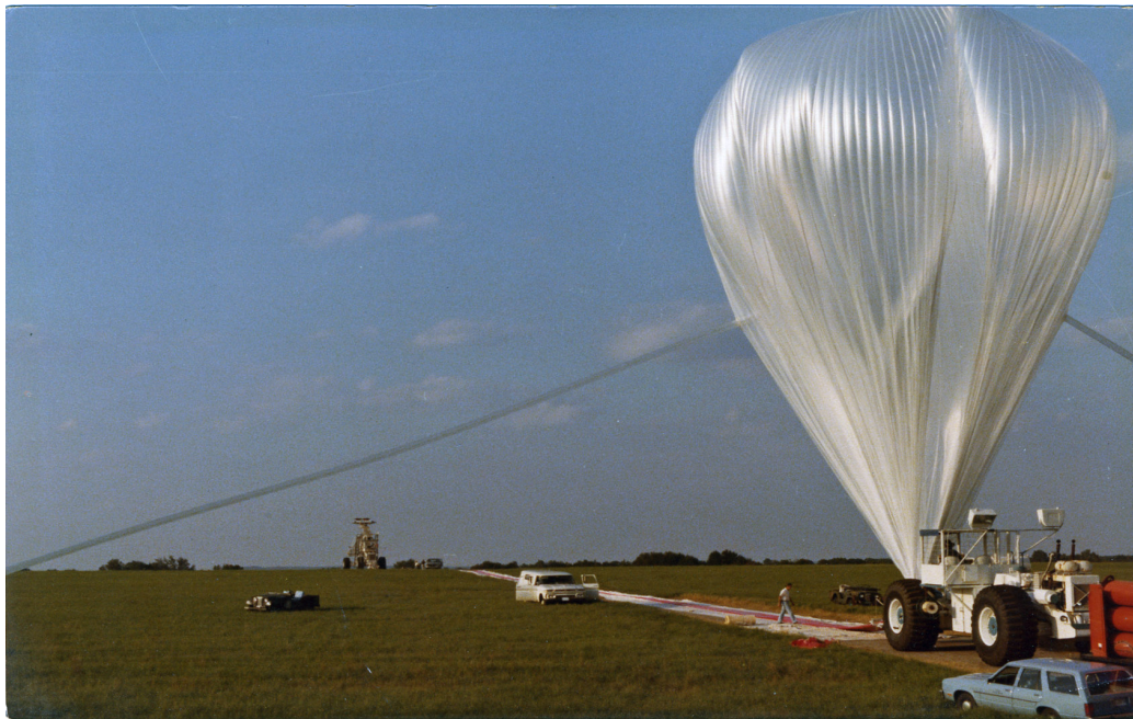
Figure 16 – The launch lay-out for the balloon parachute and payload for a typical balloon flight after inflation and just prior to launch.
